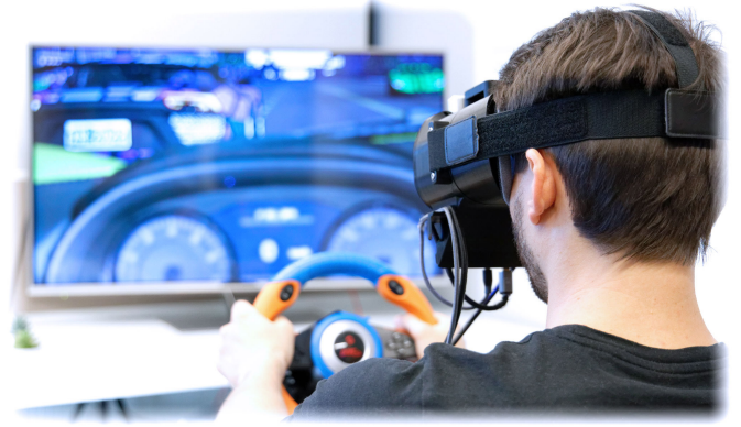
Fig. 7. A photograph of a user interacting with a two-layer display, where the first layer is displayed in a self-made head-worn prototype, and the second layer is a large passive-stereo TV set in the background.
