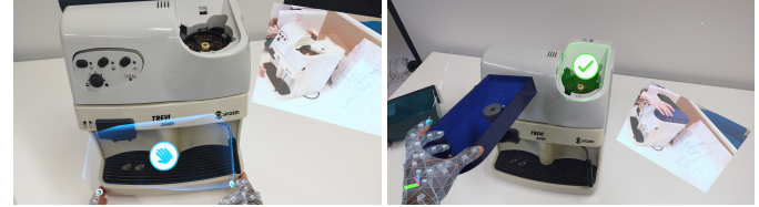
Fig. 8: The guidance mode visualization in first person view as shown on the Hololens 2: On the left, a part is in todo state, and on the right side, a part is in correct state, as a result of the interactive guidance detecting a correct assembly step.
