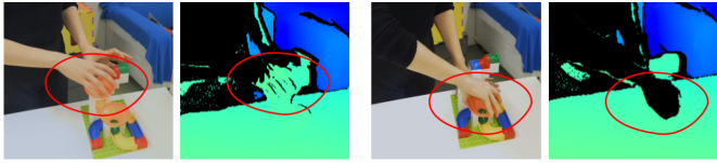
Fig. 4: Under- and over-segmentation of the user’s hands – the body segmentation sometimes has challenges around the depth discontinuities of the body. While a too large mask is not a problem, an under-segmentation can lead to noise in the reconstruction, as small hand areas can be wrongfully integrated.
