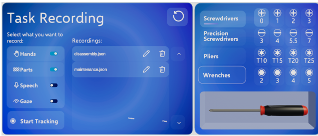
Figure 3: The Task Recording menu (left) allows the user to select what information to record and provides a button to start and stop recording. Saved recordings can be accessed from the list on the right. While recording a task, the expert operator can select a tool from the tool menu (right) and demonstrate its usage.
