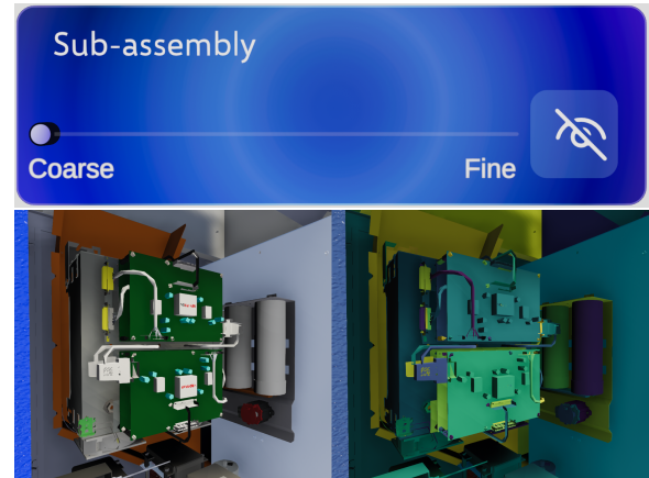
Figure 4: Using the sub-assembly slider (top), users can manipulate different levels of the parts hierarchy. Parts can be highlighted to increase contrast and to identify other parts in the same sub-assembly. (bottom)
