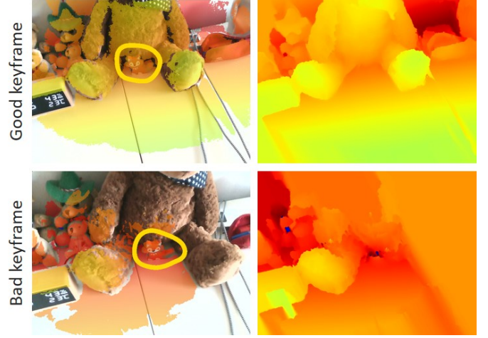
Fig. 8. “Reconstruct the scene fully” (rule 6). The top and bottom rows show good and bad keyframes with respect to rule 6. The left column shows keyframes with a SLAM reconstruction overlay. SLAM needs to explore the scene to collect sufficient depth samples. Note that pixels that have not been covered by SLAM are fully filled with a diffusion-based inpainting algorithm [32] before running the main depth inpainting [15]. However, real observations are more reliable than the convoluted depth taken from adjacent pixels.
