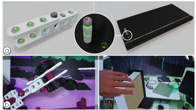
Figure 3: Mounting points and example data. (a) Mounting points (in green) on an object in a particular state. The mounting points can be in holes as well as, for example, on top of a pin, or on the object surface. (b) Samples from our synthetic datasets.
