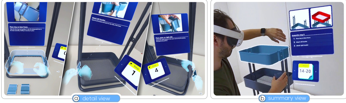
Figure 1: Adaptive AR instructions provide (a) a detailed view, showing each procedural step using AR hand animations and, optionally, a video demonstration on a virtual billboard, and (b) a summary view, presenting a summary visualization of recurring actions or action groups. The system presents the detailed view the first time an action occurs and the summary view thereafter. From the summary view, users can interactively request the detailed view of a single action in case more guidance is needed.
